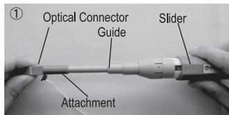
② Cleaning ends when the slider is pushed all the way. When pressure is relieved the slider naturally returns to its starting position, ready for the next cleaning. Remove the connector from the attachment to end the cleaning process.
